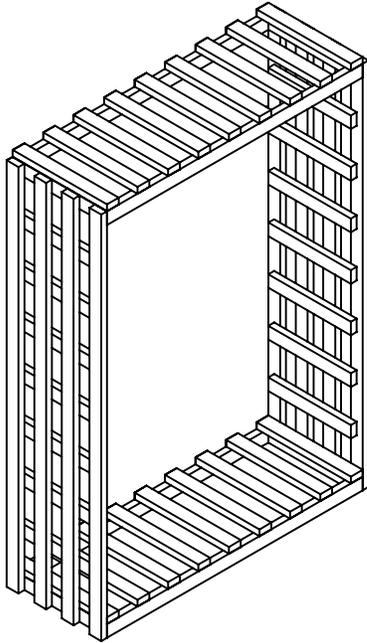
2. Nail only the bottom shelf to the side rail. Leave the top shelf to keep the spacing.
