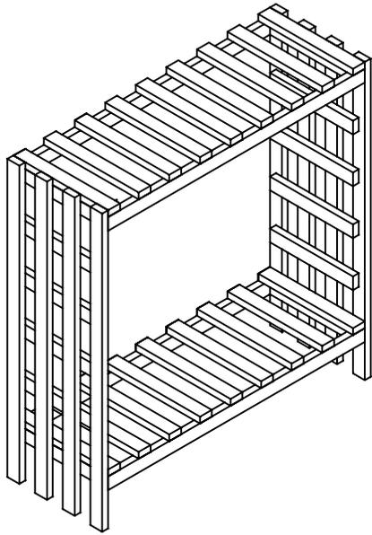
2. Nail only the bottom shelf to the side rail. Leave the top shelf to keep the spacing.
